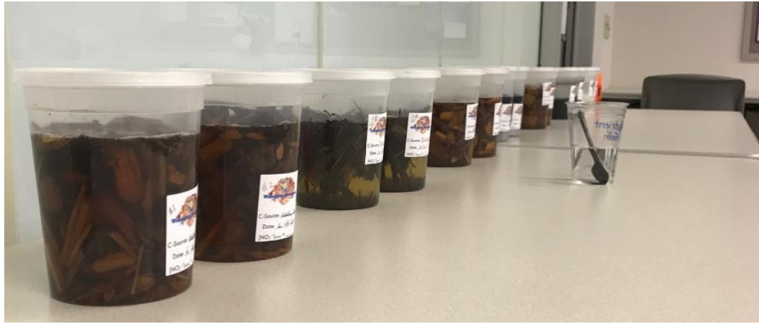
Photo of bioreactor setup in 1-quart plastic containers.
